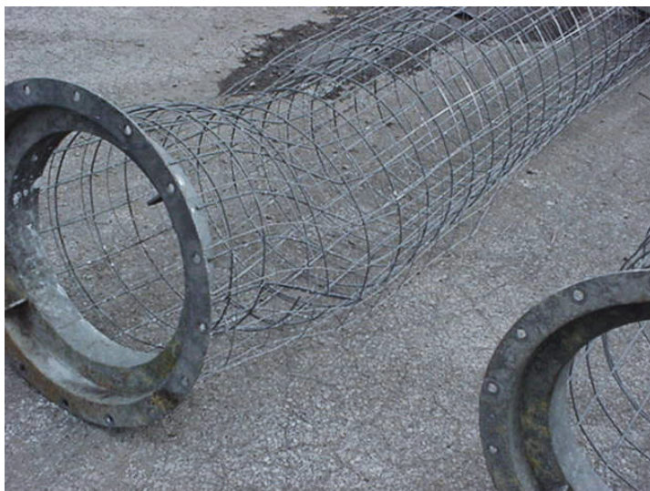
BEFORE REPAIR AND PREPACK - Mishandling of this fiber bed has caused serious damage to the cage and flange of this stripped element.
